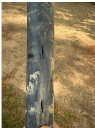
Cracked pipe causing leak on Nut Hatch Rd.
